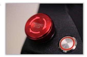
feed will not operate after the E-Stop is released if the direction handle is either in the left or right position. The direction handle must be returned to the neutral or off position, then the status LED will turn from **red** to **blue** letting you know you can now operate the power feed either right or left direction.
