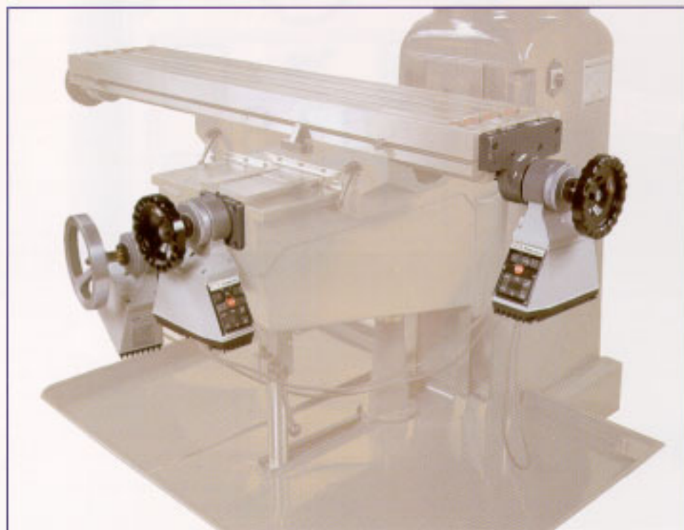
SERVO TURBO DRIVES mounted on the table, cross and knee of a Lagun Deluxe mill. (Machine courtesy of Republic-Lagun, Carson, CA)
