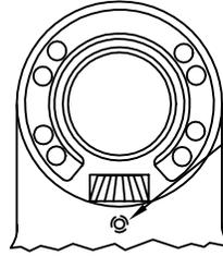
TIGHTEN SLIGHTLY (HOLDS BEVEL PINION STATIONARY DURING SHIMMING.)
